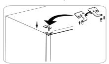
15. Remove the upper hinge cover from the plastic bag provided, and install it and fix it with screws.
