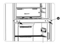
9. Lay the refrigerator on soft foam packaging or similar material. Remove both adjustable bottom feet parts, and the lower hinge part by unscrewing the special flange self-tapping screws. Loosen the lower hinge axis then install it on the reverse hole site.
