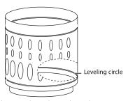
Add water to the washer until it reaches the leveling circle. If the washer is level, the water will touch the leveling circle all the way around. If it's not level, it will only touch part of the leveling circle.
