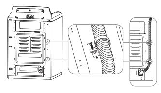
5 Position the other end of the drain hose (the loose end) in one of the following ways:
