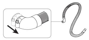
2 Insert the drain hose with the clamp onto the washer's drain pipe. Make sure that the drain hose completely covers the end of the drain pipe.
