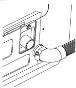
3 Move the clamp toward the drain pipe outlet. Tighten the clamp with a flat blade screwdriver.
