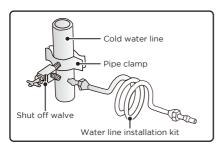
The minimum inlet water pressure: 147KPa The maximum inlet water pressure: 834KPa
